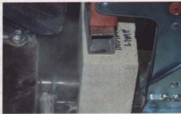
Ultra-high speed drilling test at 50,000 rpm in limestone. (Photo courtesy of DOE)
